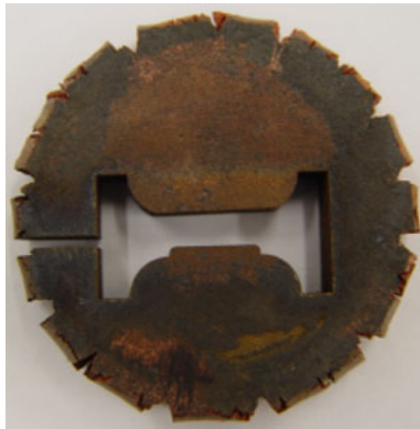
Fig. 8 The Cu disc produced by powder compact forging (the image also shows the location and shape of the tensile testing specimens cut from the forged disc)
